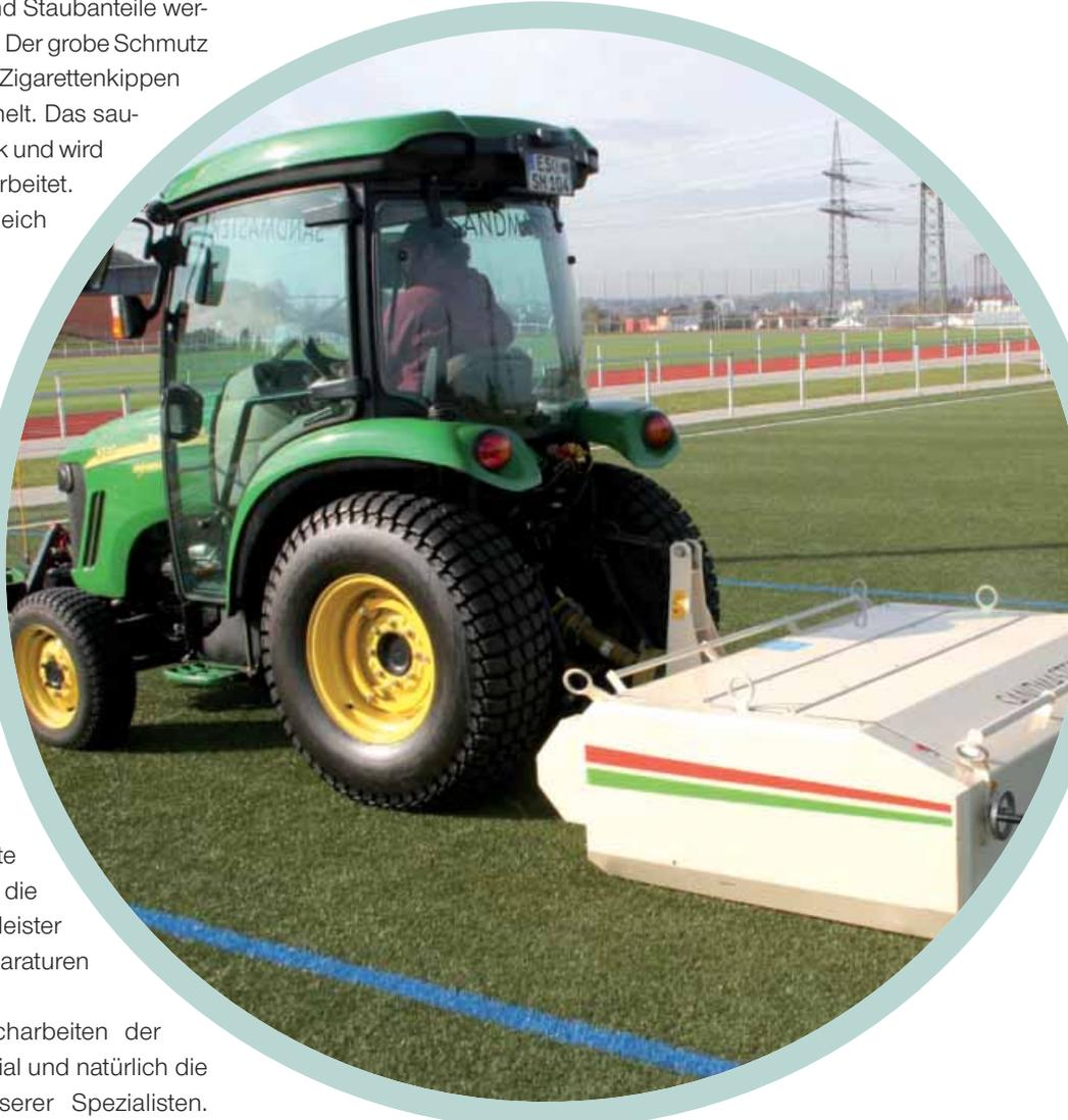
*pile and suction-cleans it of dust and fine dirt which is collected in nonwoven filters. Coarse dirt such as stones, glass fragments, chewing gum, cigarette ends and leaves are sieved out and collected. The clean filler material is then returned to the pile and "settled in" by a roller brush. At the same time, bent turf stalks are straightened again.*
